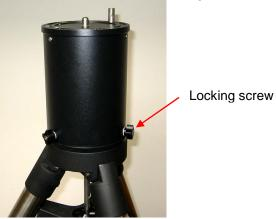
4. Final adjust the tripod height and level the tripod with MiniPier before mounting the iEQ45 mount.
